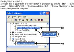
1) "FX-USB-AW/FX3U-USB-BD" is displayed at A), as part of the list of the "Universal Serial Bus controllers".
